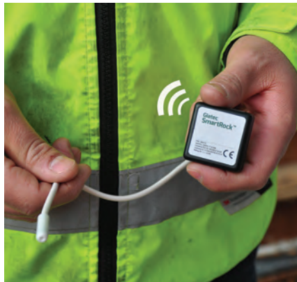
ABOVE AND LEFT: SmartRock is a rugged, mobile-based wireless sensor that is fully embedded in fresh concrete to monitor its in-place temperature and strength during construction.
