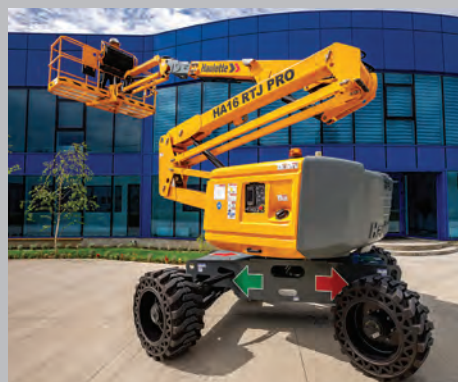
LEFT AND BELOW: Haulotte HA16 RTJ Pro articulating boom is fitted with Haulotte's Activ'Screen, Activ'Lighting System, Stop Emission System and Activ'Shield Bar.
