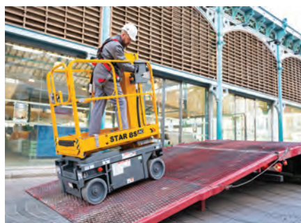
ABOVE AND RIGHT: Haulotte's new Star 8S vertical mast is designed for indoor use, offering a load capacity of 200 kg and travel speed of 4.5 km/hr.
