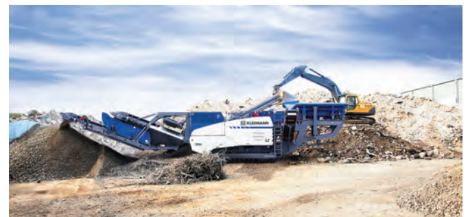
Mobirex MR 130 Z EVO2 impact crusher from Kleemann.
