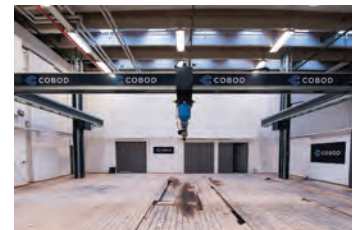
The BOD2 3D construction printer being tested before shipment.
