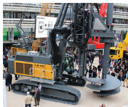
RIGHT AND BELOW: The new LB 45, the successor to the LB 36, features a torque of 450 kNm, an increase of about 10%.
