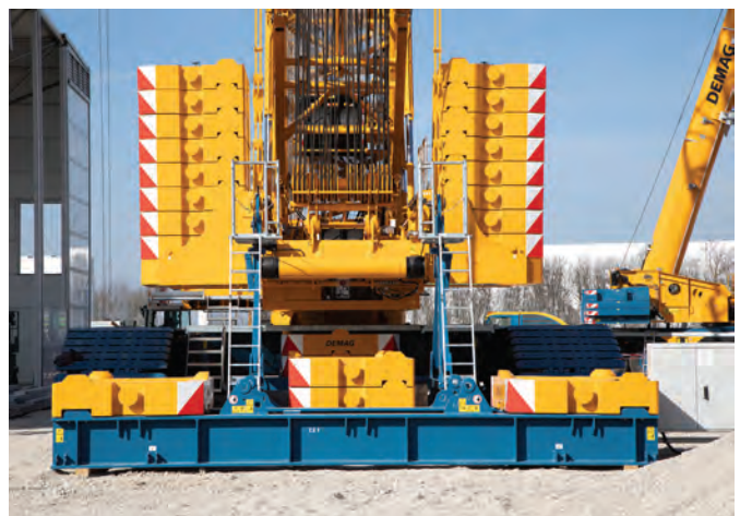
TOP AND ABOVE: The new Demag CC 2800-2 lattice boom crawler crane, the successor to the CC 2800-1 model, offers a maximum lifting capacity of 600 t and maximum load moment of 7,712 tm.
