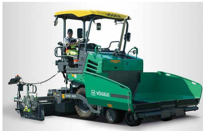
ABOVE AND LEFT: Vögele has developed two new compact pavers, as part of its Classic Line. These include the Super 1000(i) tracked (above) and Super 1003(i) wheeled (left) pavers.
