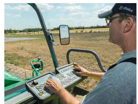
BELOW: The Niveltronic Basic system for automated grade and slope control has been integrated into the machine control system.
