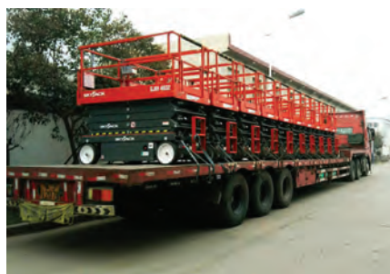
Skyjack SJIII 4632 DC scissor lift has a maximum working height of 11.58 m and 204 kg capacity. It can lift and lower in under 60 seconds.
