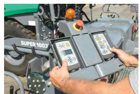
The new compact pavers are equipped with the ErgoBasic operating concept.
